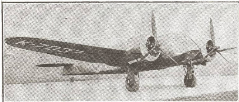
Under the British term "medium bomber" this Bristol Blenheim, now being supplied to the Royal Air Force in large numbers, is vaunted by the Englishers as the fastest machine of its class in the world. A low-wing, full cantilever job, the Blenheim is powered with two Bristol Mercury engines. It has a service range of well over 1,000 miles and an official top speed of 279 m.p.h. Indeed, some reports have it that the Blenheim can do 285 m.p.h. at 15,000 feet! Observe the "frog-nosed" prow of the plane, also its sturdy retractable undercarriage.
