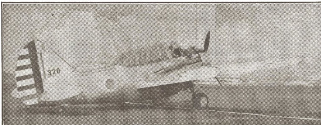
Left: Some of our National Guard flyers are getting fine training aboard North American jobs of this O-47 type. The true performance figures of this sturdy three-place observation craft are still "hush-hush," but it is believed to be very fast for combat tangles and suitably slow when artillery co-operation work is on the bill.
